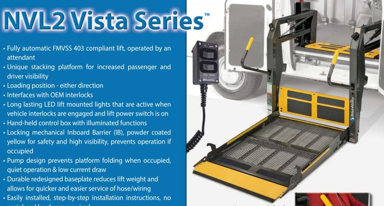
Integrated dual handrails provide added security for wheelchair users and standees
